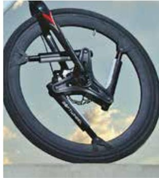
**39** Israel has literally reinvented the wheel. The Softwheel is the brand name given to a wheel with a flexible shock absorption system built into the wheel itself. It boosts stability without sacrificing speed - in wheelchairs, bikes, cars and even planes.
